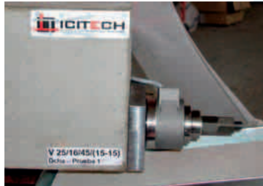
Fig. 5: C6A 200 kN force transducer for measuring external anchoring forces
