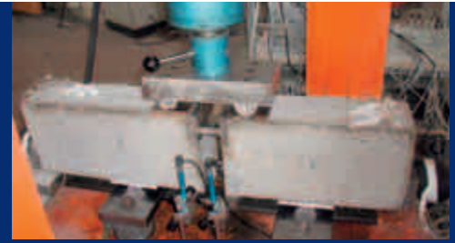
Experimental analysis of mechanical stress in passive reinforcement anchorages in C-C-T nodes
