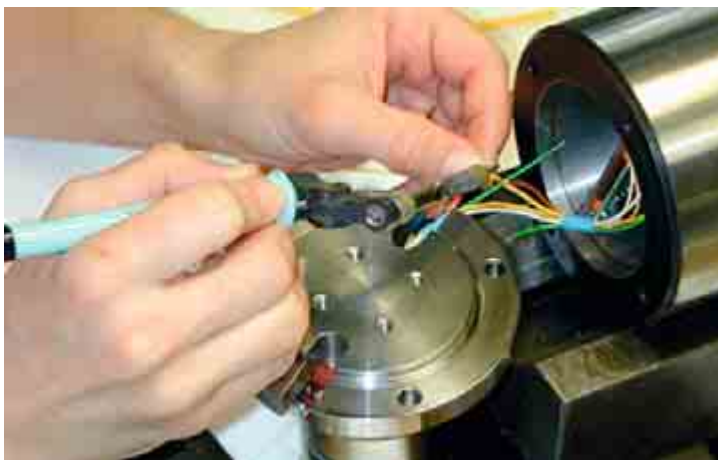
Fig. 10: Slip ring transformer installation
