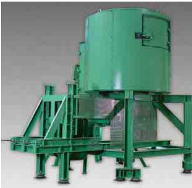
Fig. 1: Recycling machine for separating compounds; on the right, the test version
