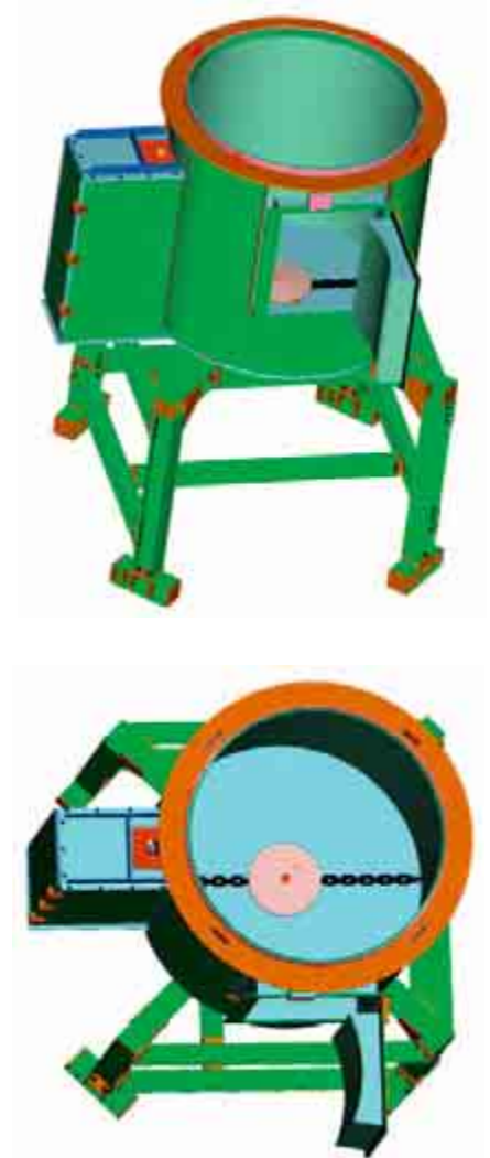
Figs. 2a, 2b: Recycling machine without the drive (CAD drawing)
