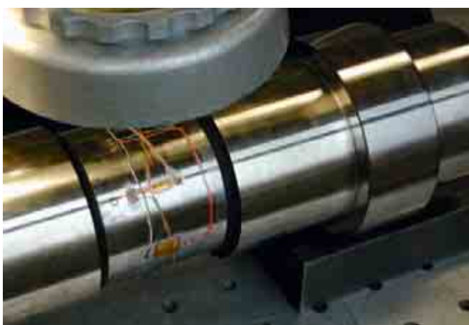
Fig. 5: SG installation and wiring on the input shaft, SG full bridge (torsion), 2 SG half bridges (bending on two axes)
