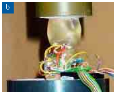
Fig. 2: Test setup and teeth models with SGs for investigating the anterior (a, b) and lateral (c, d) teeth groups in accordance with the load schemes in Fig. 1
