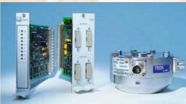
Predestined for the measurement chain: U10M force transducers in a double bridge version, the TEDS module is integrated in the transducer housing. Next to this, TEDS-compliant multi-channel modules using carrier frequency technology for the MGCplus amplifier system: ML455 amplifier module with an AP455i connection board
