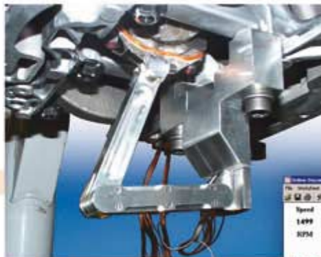
Fig. 3: Fully installed piston telemetry system
