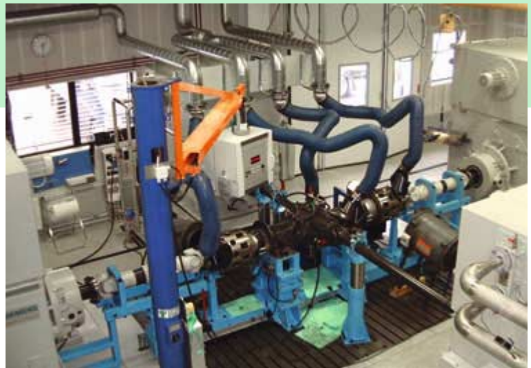
Fig. 2: Test rig with rear axle transmission as a test specimen
