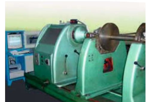
Fig. 3: Balancing machine after conversion
