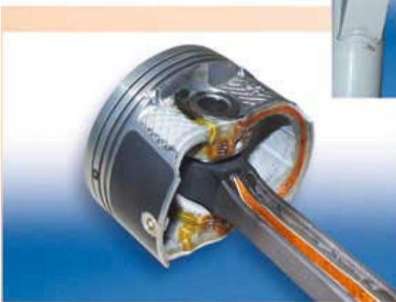
Fig. 2: Eight thermistors are placed under the combus- tion recess of the piston
