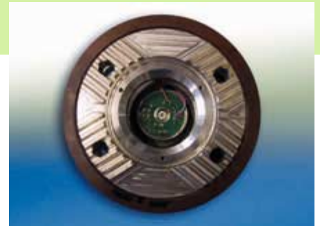
Fig. 5: To prevent unbalance, the rotor electronics are mounted centrally
