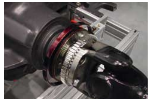
Fig. 1: Torque transducer: mounted between the rear axle and the cardan shaft
