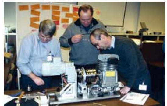
Fig. 2: "Measuring torque correctly" seminar, workplace no. 1: Mounting a torque flange
