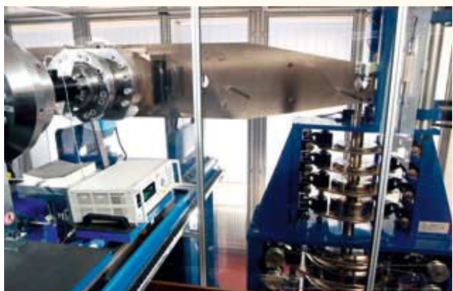
Fig. 1: It always was good, but now it's even better: Torque calibration at HBM
