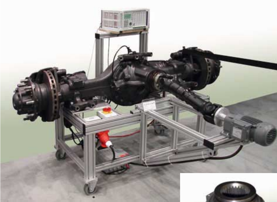
Fig. 2: Truck rear axle with torque transducer
