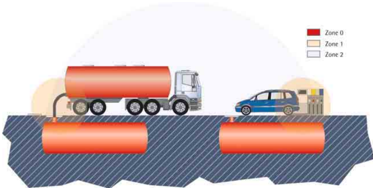
Classification of hazardous areas into ATEX zones using a fuel station as an example
