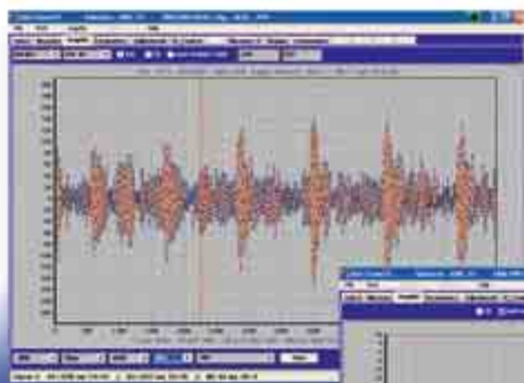
AEDpanel32: Unfiltered signals from an operating checkweigher
